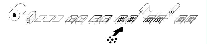
**THERMOSEALER** Todays packaging line world is divided into either thermoforming or tray sealing lines, the first producing value packs, the second higher quality packs with greater flexibility.
